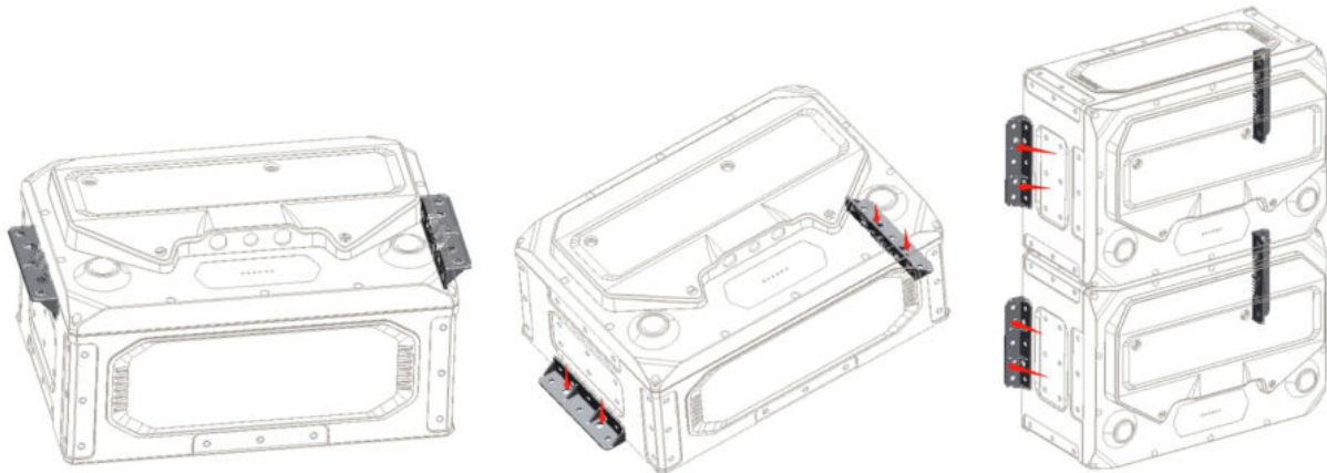
Figure 3: HUSKY2 Mounting Installation
