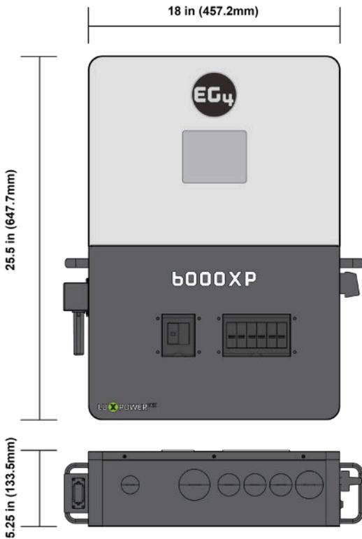
The 6000XP is a 208/240 VAC split-phase, 48 VDC off-grid inverter/charger capable of utilizing 8kW of PV and efficiently outputting 6kW of power while also charging the battery bank.
