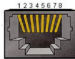
Figure 7: RJ45 Port of Battery
